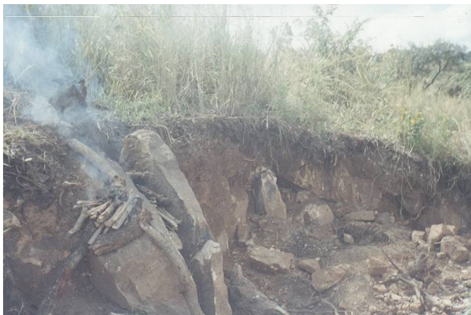
Figure 2. Quarry works on Keyo Hills. Trees in the surrounding area are cut down and the logs used for heating and weakening the stones for easy crushing.
